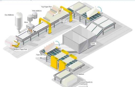
The initial materials are homogenously mixed to form a gypsum slurry that is spread via hose outlets onto a paper liner on a moving belt conveyor. A second paper liner is fed onto the production line from above to form the plasterboard. The plasterboard continues along the production line where it is finished, dried, and cut to size.
